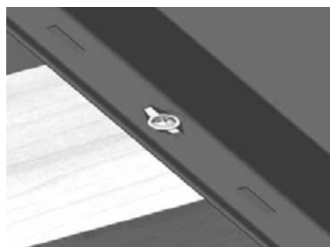
Figure 16. A screw that is too tight
