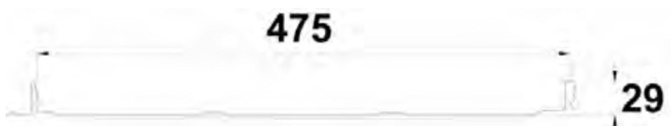
Figure 4b. PROGANTTIJ nominal cross-section dimensions in accordance with the tolerances specified in SFS EN-508-1
