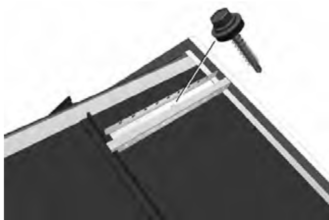
Figure 31. Fixing the Progantti ridge seal
