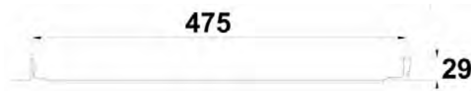
Figure 4a. PROGANTTI nominal cross-section dimensions in accordance with the tolerances specified in SFS EN-508-1
