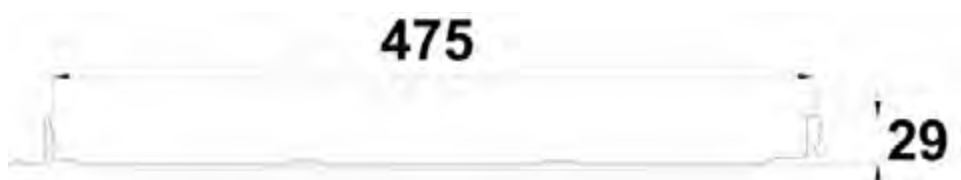
Figure 4b. PROGANTTIJ nominal cross-section dimensions in accordance with the tolerances specified in SFS EN-508-1
