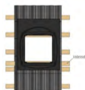
Figure 41. Add extra batten if necessary
