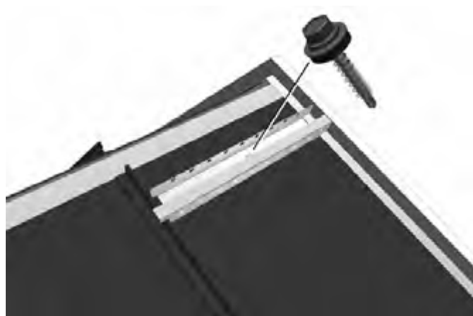
Figure 31. Fixing the Progantti ridge seal
