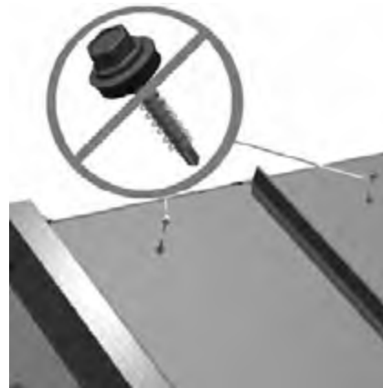
Figure 18. Do not fix the sheets to the battens from the top end with screws
