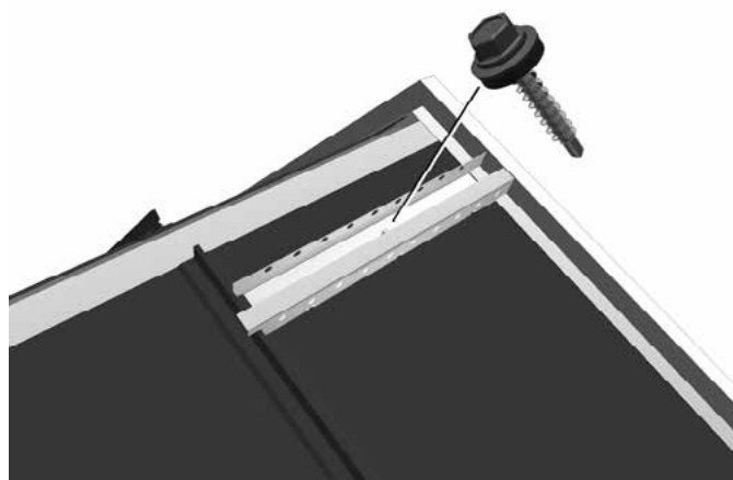
Figure 31. Fixing the Progantti ridge seal
