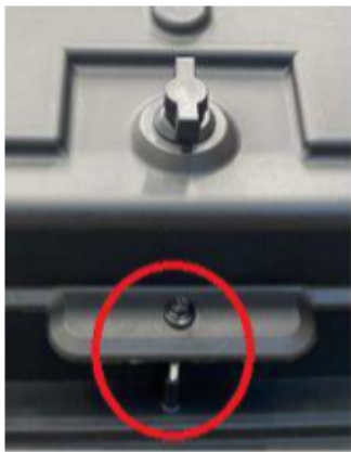
Figure 49. Hatch locked and secured with a screw
